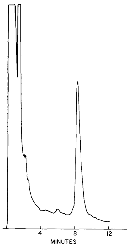
FIG. 1. GLC tracing of \alpha -tocopherylquinone ( 0.07 \mu\text{g} ) from 0.5 \text{ ml} of human red cells after TLC separation. The sample was dissolved in 50 \mu\text{l} of \text{CS}_2 , and 5 \mu\text{l} was injected. Column was 3% QF-1, 228^\circ\text{C} ; argon, 50 \text{ ml/min} ; air, 330 \text{ ml/min} ; hydrogen, 11 \text{ ml/min} ; attenuation was 9 \times 10^{-12} \text{ amp} .
